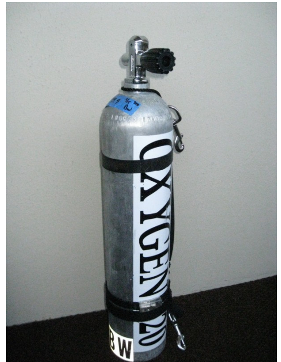
Properly marked O 2 decompression bottle. Note the analysis tape on the shoulder of the bottle, and only "OXYGEN 20" on the sides of the tank, with no other distractive stickers. The initials "BW" are at the bottom of the back of the tank, so as to not interfere with the MOD stickers.
